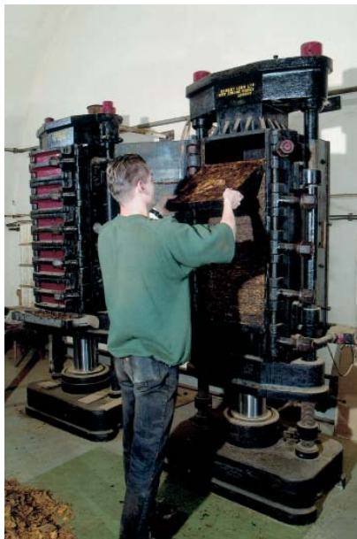
left: Our two historic heated flake tobacco presses from England. Here the fresh tobacco „cakes“ are taken from the press.
